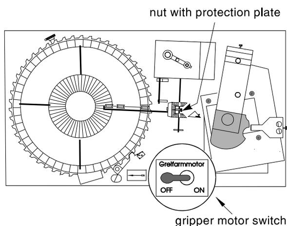
1. Gripper arm has to be in carrier position.
