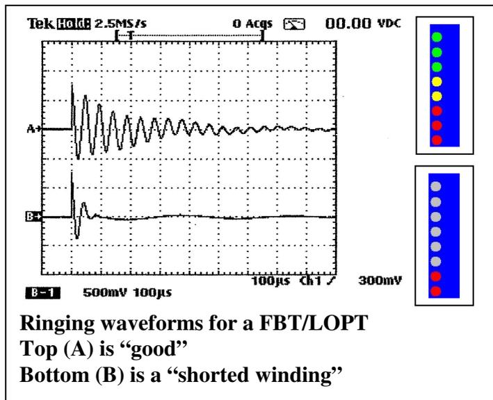
Waveform A shows the ring response to this tester's pulse for a good FBT/LOPT. Note several rings in a decaying fashion. This tester will count the rings that exceed its threshold and display them as lit LEDs as shown in the simulation to the right of waveform A.
