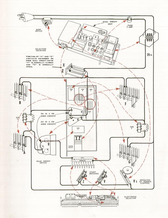
TRIP SOLENOID - Picture Diagram Select-o-matic "200" - V-200 (NOT A SCHEMATIC OR WIRING DIAGRAM)
