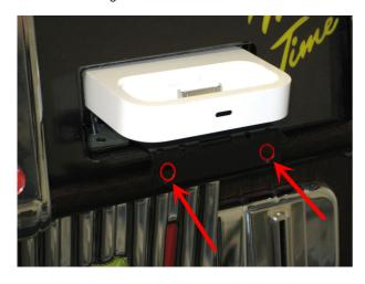
11. Mount the BGM connector (pos.1) and the power supply for iPod (pos. 2)with the brackets attached to the kit in front of the selection & credit computer.
