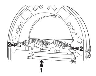
Loosen the nuts behind the keyboard and remove it to the front.A 7mm socket wrench is included in the kit.
