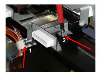
10. Pull out the docking station and mount the stainless steel plate with 2 hexagon nuts M4 from behind.
