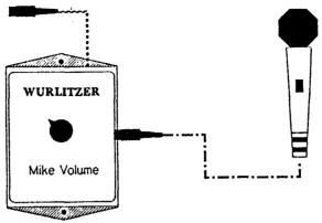
This unit enables the use of the phonograph as a paging system, when playing as well as during idling periods. If the paging microphone is switched on while the phonograph is playing, the music fades away for this period. The volume of the microphone is adjustable at the pre-amplifier box. A cable length of 15 meters (approx. 50 feet) allows to install this kit in distance to the jukebox.
