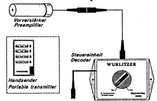
With this wireless RVC four basic functions can be controlled over a portable transmitter: increase of volume decrease of volume
