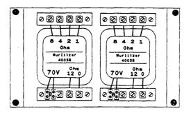
For connection of an external loudspeaker to match its impedance or volume. Also 70V loudspeakers are connectable.
