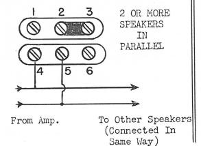
NOT USING MATCHING TRANSFORMER (Use fader adapter with Model 1015 or 1080 Phonographs)
