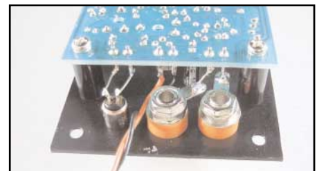
Fig.11: The front panel is mounted between the plastic collar and ring of the banana socket. Then two nuts are used to hold and lock the assembly in place.
